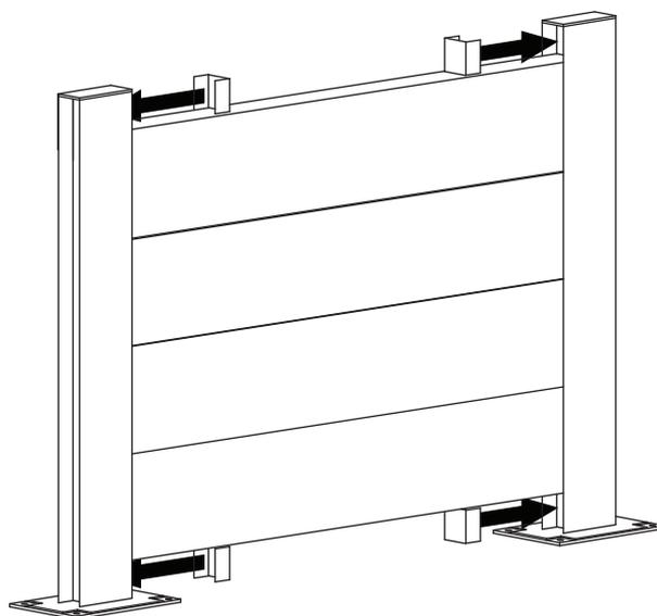
7. Fixer le platine au sol (Vis 5,5x50, Cheville 9x50, Rondelle et Bouchon)(
